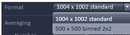
Fig. 115 Format drop down menu – appearance for WF, SIM and Laser WF imaging modes
