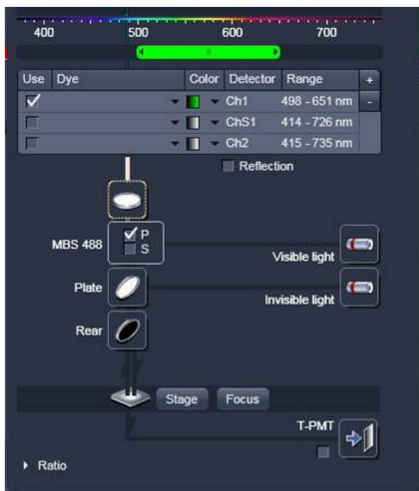
Fig. 625 Light path with Notch filter cascade option
