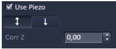
Fig. 163 Use Z-Piezo stage for Z-Stack acquisition – appearance for the LSM imaging mode
