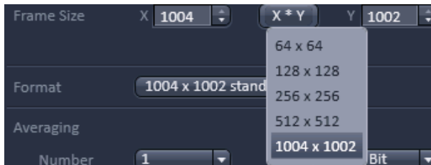
Fig. 114 Frame size drop down menu – appearance for WF, SIM and Laser WF imaging modes
