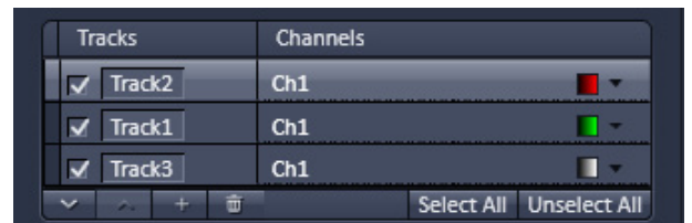
Fig. 139 Track selection display – Track 2 moved to the top, no further upwards movement possible
