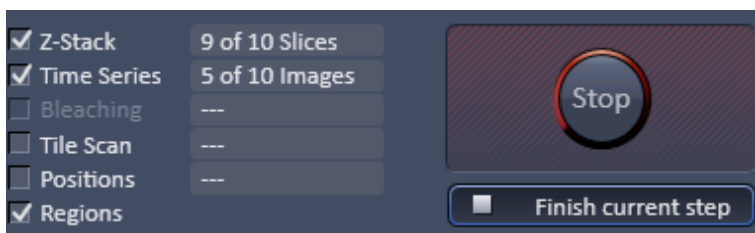
Fig. 82 Multidimensional input field – display of the current status 9 from 10 slices taken from the 5th of the 10 images
